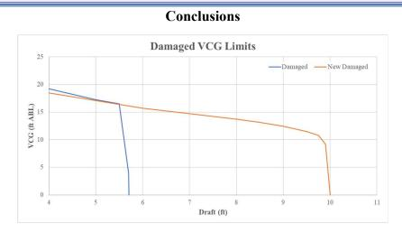
The *Lilac* can be modified to comply with small passenger vessel (Subchapter T) stability regulations in the Code of Federal Regulations. Her displacement should be limited to 927 LT or less, and the vertical center of gravity of her loading condition must not exceed the value on the maximum VCG curve for a given displacement.
