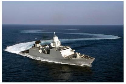
Zig-zag test on LCF frigate of Dutch MoD (www.dutchdefencepress.com)
