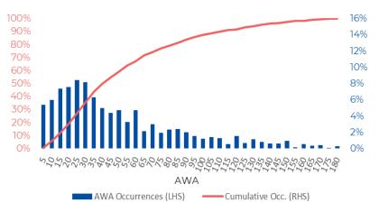
> 79% of the wind sailing conditions of the ship will be below 75° of Wind Apparent Angles.
