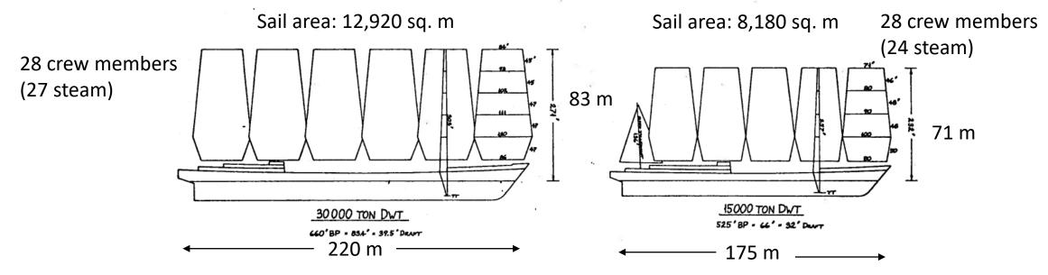
**Result of 1975 MARAD Study**: bulk cargo ships sailing vessels had a higher required freight rate (RFR) than engine-driven vessels.
