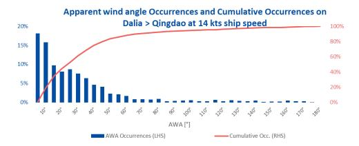
> Oceanwing is the most relevant wind propulsion technology as more than 80% of the apparent wind angles are below 45°.
