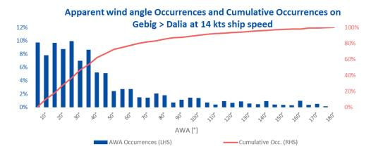
> Oceanwing is the most relevant wind propulsion technology as more than 67% of the apparent wind angles are below 45°.
