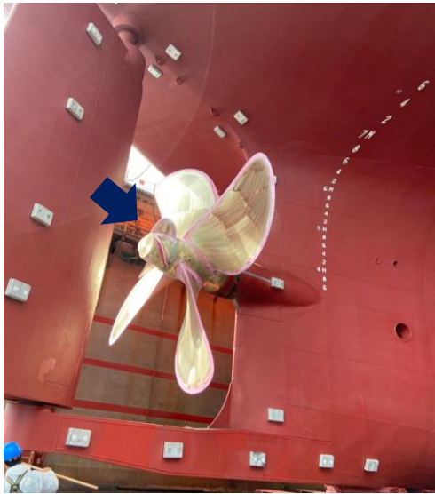
A high-performance hull coating was applied to Octonaut and a PBCF was retrofitted in June 2022. Other ESDs will be retrofitted on the vessel whilst in service
