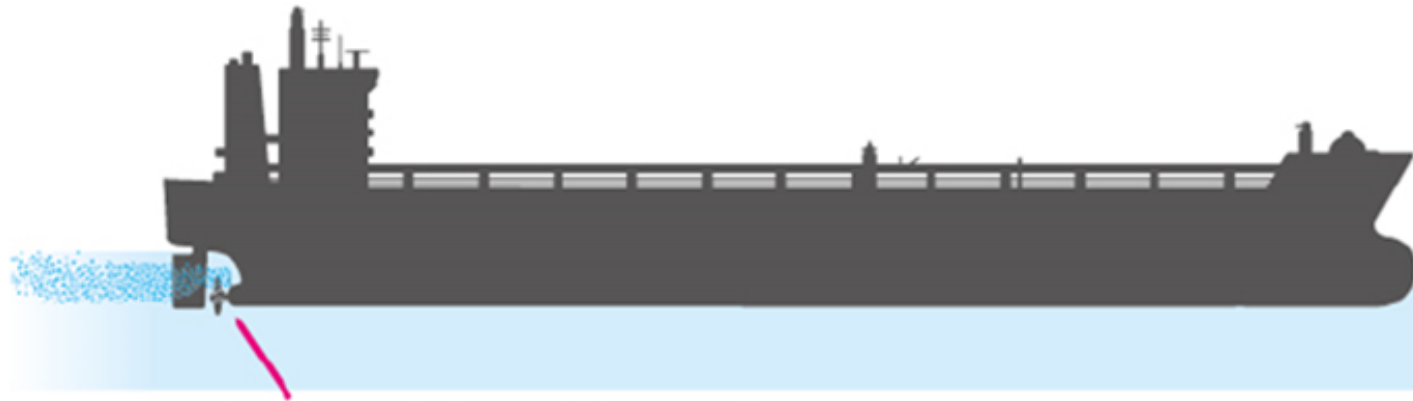
Bubbles injected in propeller inflow
