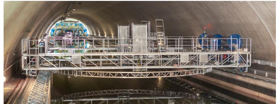
Model-scale noise measurements in Depressurised Wave Basin using silent towing carriage
