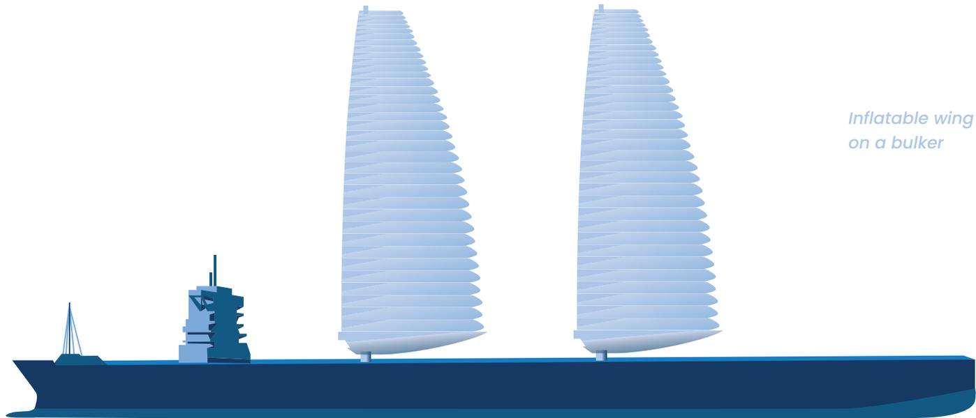
*Inflatable wing integrated on a bulker*
