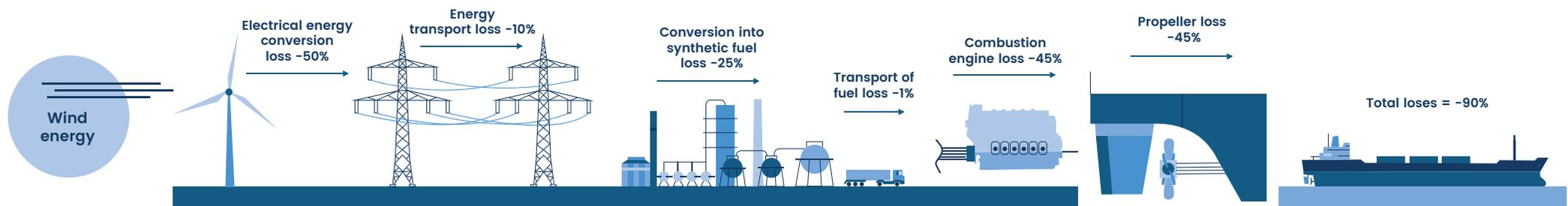
Theoretical diagram of the production of a synthetic fuel from wind energy to power a ship
