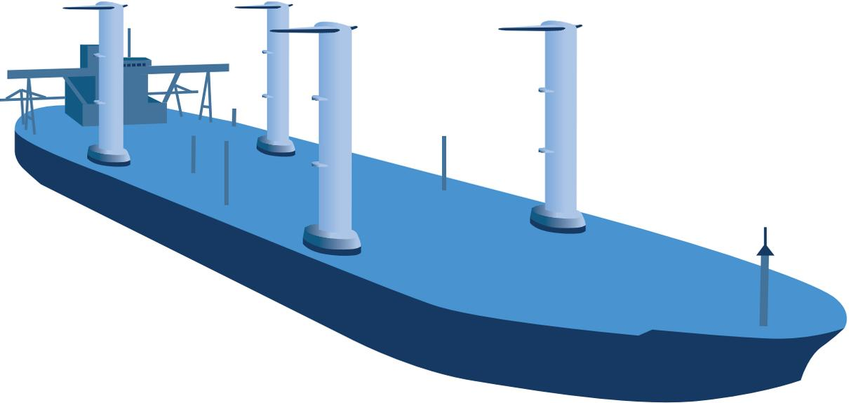
*Suction wing integrated on a tanker*
