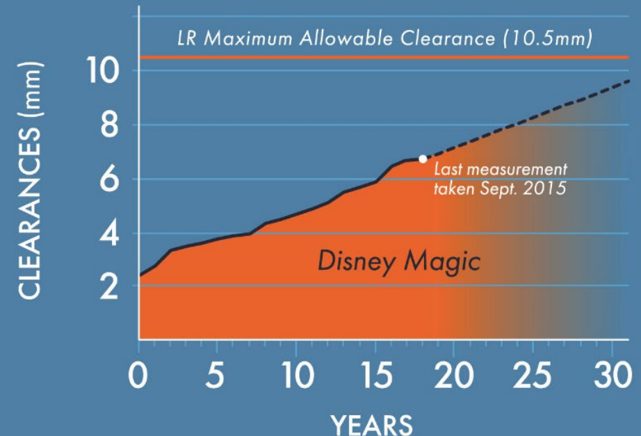
Thordon COMPAC Water Lubricated Propeller Shaft Bearing Clearance (Avg. Clearance of Port & Starboard)
