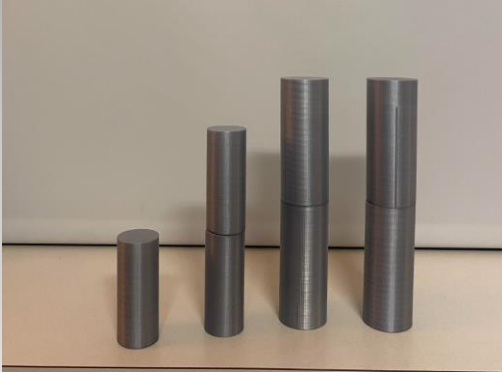
3D-printed rotors, singular, 10/3.8 cm and stacked 20/3.8 cm and 25.4/5.1 cm
