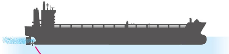
Bubbles injected in propeller inflow
