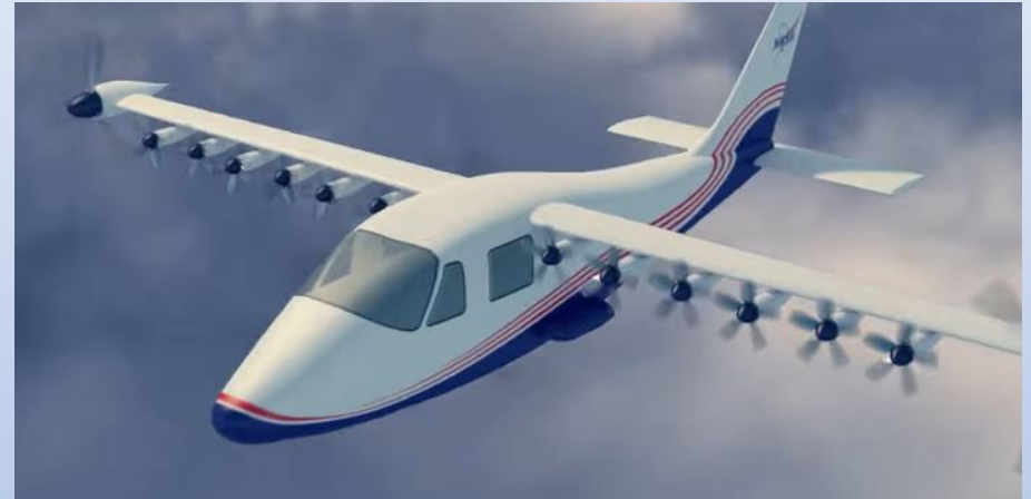
NASA X-57 with distributed electric motors and contra-vortex propellers on wingtips
